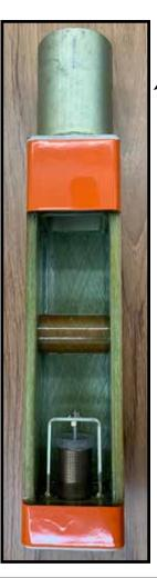
Cut away view shows interior construction including moisture removing desiccant canister and bonded in place pin bosses
