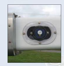
Desiccant Canister: Moisture in the sealed jib is detected in the desiccant canister and is visible from the ground when the IWP is working, stowed, covered or uncovered.
