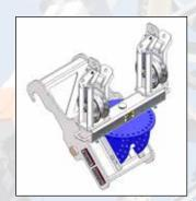
Bundle Lifter: Can lift 2 conductors, up to 2500 lb (1134 kg) each. Rotates 180°, and adjusts to jib angles from 35° to 80° in 5° increments. Can be replaced by a single conductor lifter with a capacity of up to 5000 lb (2268 kg).
