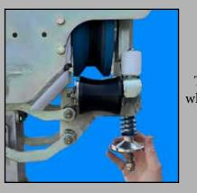
Tighten the adjustment wheel if the rubber-coated wheels are slipping.
