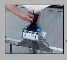
Drive control is placed for easy use. The 3-position toggle switch controls 2 wheel rear drive, 4 wheel drive, or 2 wheel mid drive.
