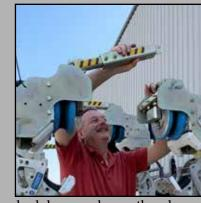
Top lock bar can be easily released and the wheels and motors moved to make it easy to put the cart on the line.
