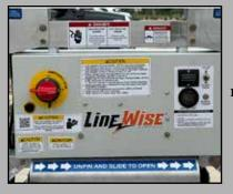
Main control panel has a distance counter, main battery disconnect and lithium battery on/off switch.
