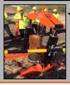
Stub Puller option allows removal of poles that have been cut off above ground level, but at a height too low to pull out with the standard Pole Puller. Pole Puller successfully removes poles that are foamed in rocky soil!
