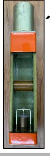
Cut away view shows interior construction including moisture removing desiccant canister and bonded in place pin bosses
