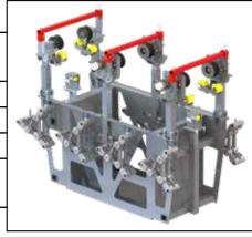
nd 2x composite idlers plates, insulators & spacers Center main wheels raise/lower so each set of main rollers can be removed from conductors Wheel drive diameter = 6" (152 mm) Dynamic provided by electric drive system Braking Aluminum Alloy; Welded & Bolted Construction Occupancy 1 Person
