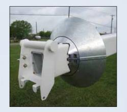
Corona Ring: The high performance, sharp-edge corona ring reduces current leakage and is rated to 500 or 765kV. Easily removeable, protective jib and corona ring covers guard against damage during transport.
