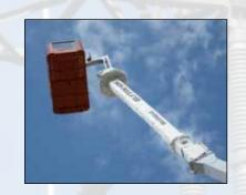
Insulated Jib: By insulating a non-insulated, telescoping crane or derrick, the need to purchase a dedicated, insulated aerial lift to perform bare-hand maintenance work is eliminated.
