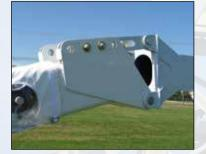
Jib Articulation: Unique slot-link adapter at crane enables pinning at ground level and lifting into position.
