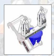
Bundle Lifter: Can lift 2 conductors, up to 2500 lb each. Rotates 180°, and adjusts to jib angles from 35° to 80° in 5° increments. Can be replaced by a single conductor lifter with a capacity of up to 5000 lb.
