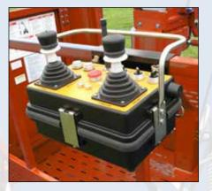
Basket Controls: Fully proportional radio controls provide operation of telescope, boom and rotation functions enabling the operator to better position the platform for the work being performed.
