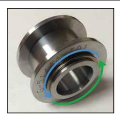
Bushings are made from heat treated 17-4 and 416 stainless steel. Different grades of stainless are used to prevent galling that takes place when "like" materials are in contact with each other while moving or through vibration.
