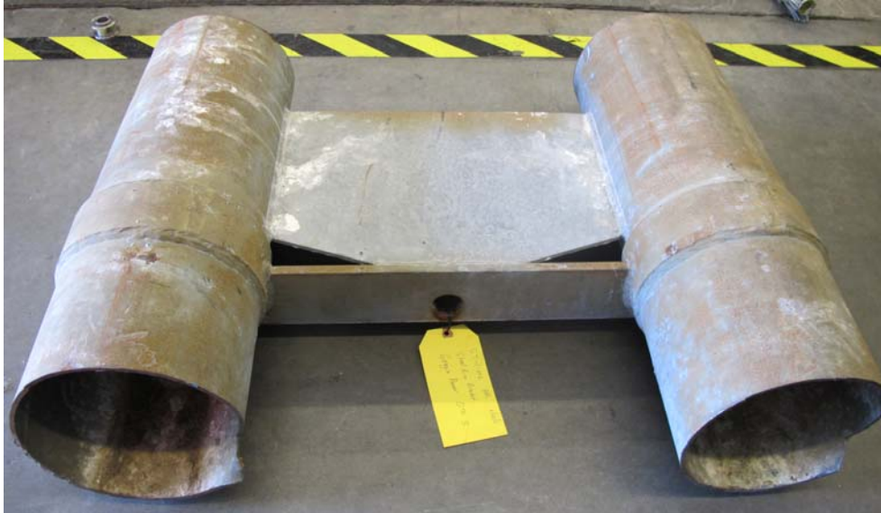
Figure 2: The as-received condition of Sample 1-2. The bushing was removed to show the condition of the eye.
