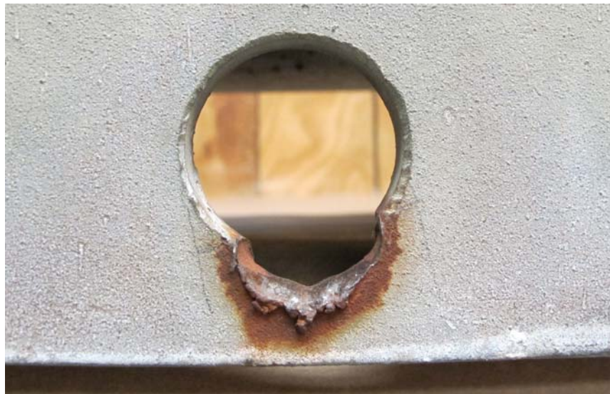
Figure 9: The as-received condition of the eye of Sample 1-3. The material appears to have yielded as there is an excess of material displaced at the edge of the wear of the eye. The wide area of the wear suggests that the Y-bolt may have been rocking and swaying over an extended period of time in the field.
