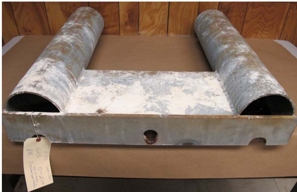
Figure 3: The as-received condition of Sample 1-3. The Y-bolt was removed to show the condition of the eye.
