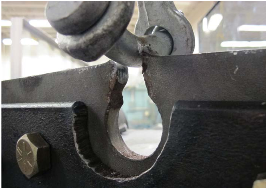
Figure 12: Sample 1-3 failure and shear tear out from Y-bolt.
