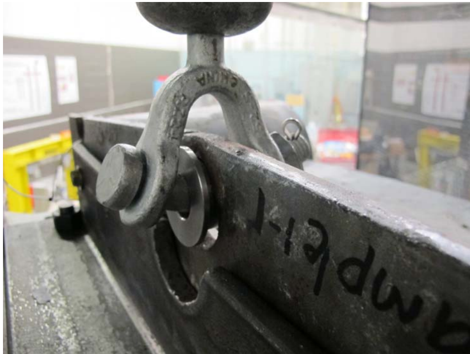
Figure 10: Sample 1-1 deformation after shear of inside bolts of fixture. The eye deformed but did not shear.
