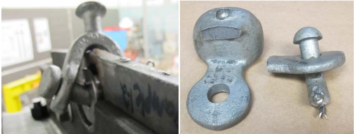
Figure 11: Sample 1-2 deformation after failure of socket of Y-bolt and a close-up of socket failure. The eye of the sample deformed but did not shear.
