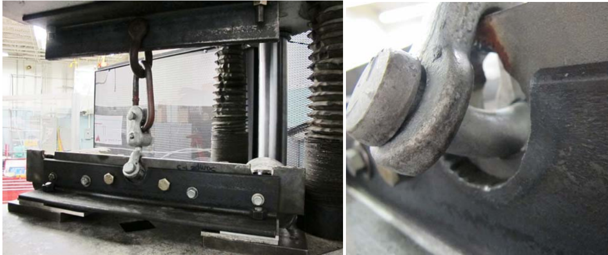
Figure 6: Test setup of Sample 1-3 and a close-up of the Y-bolt in the eye.
