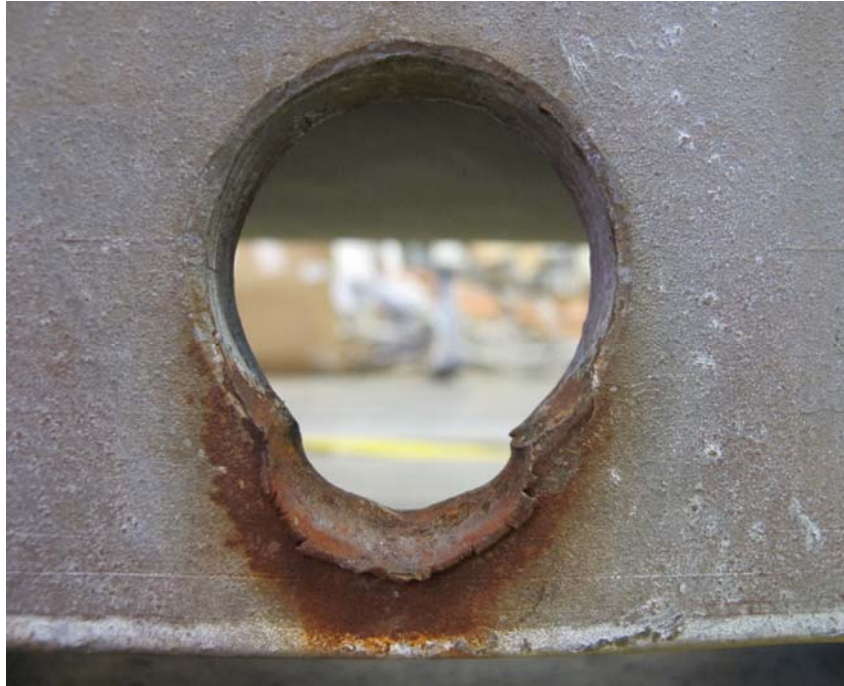
Figure 8: The as-received condition of the eye of Sample 1-2. The material appears to have yielded as there is an excess of material displaced at the edge of the wear of the eye. The wide area of the wear suggests that the Y-bolt may have been rocking and swaying over an extended period of time in the field.
