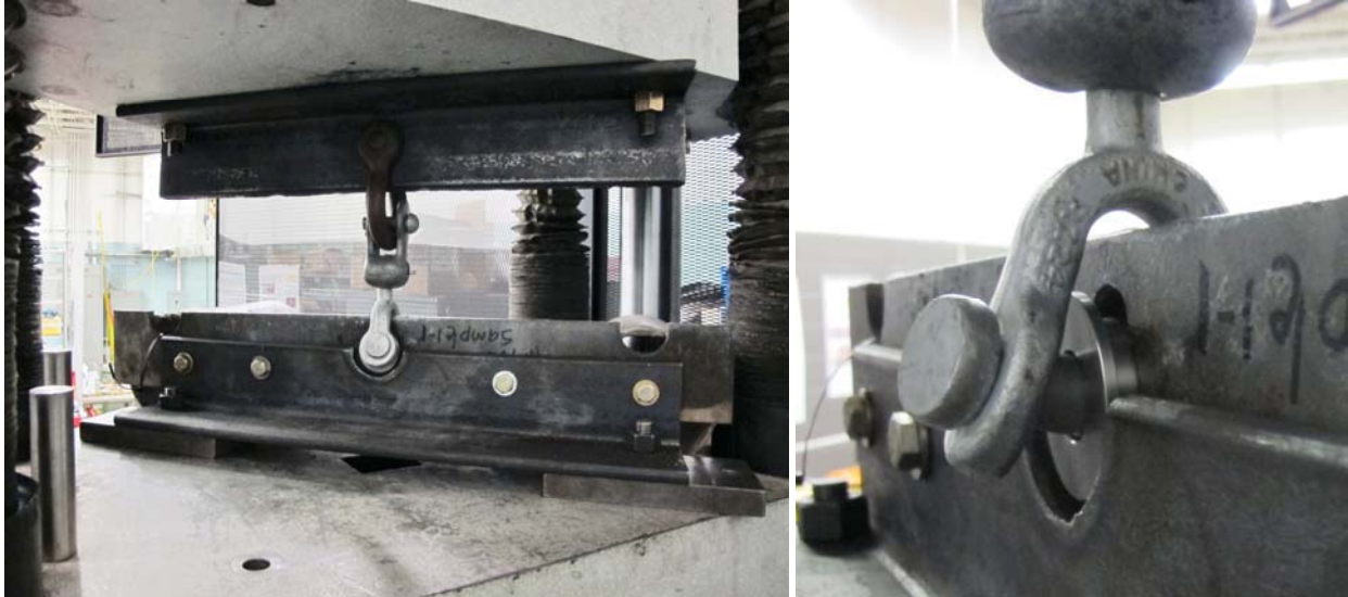
Figure 4: Test setup of Sample 1-1 and a close-up of the bushing and Y-bolt in the eye.
