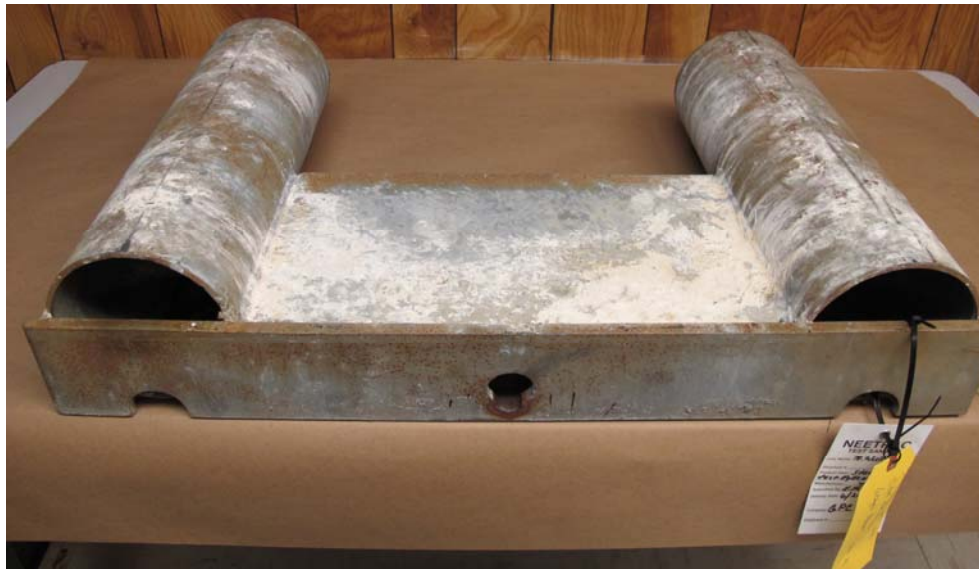
Figure 1: The as-received condition of Sample 1-1. The bushing was removed to show the condition of the eye.
