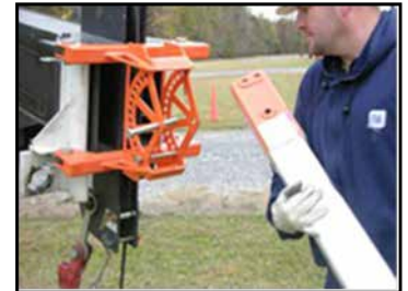
Installation of Jib
